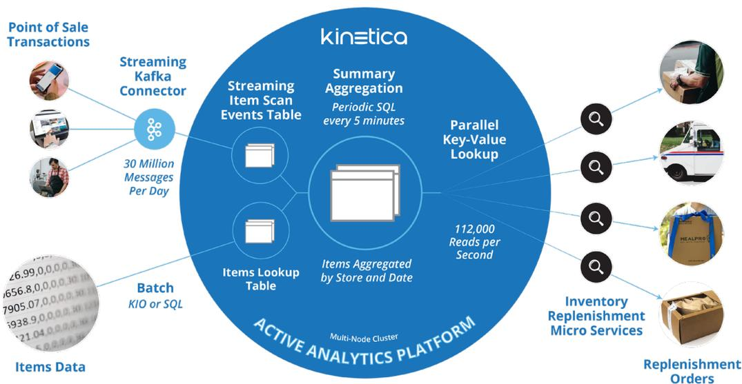
Kinetica consolidates the hardware sprawl from previously attempted solutions by powering workloads for streaming analysis, historical analysis, location intelligence, and machine learning on a single, unified platform. The Kinetica-based microservice architecture delivers high concurrency query throughput and provides a REST microservice that will enable the retailer's machine learning experts to deploy various algorithms and build on top of Kinetica as a platform.
