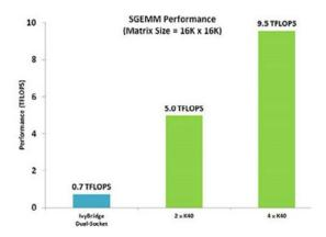
GPUs are able to scale up performance in a nearly linear manner, as shown by these single-precision floating general matrix multiply (SGEMM) benchmark tests. (Source: NVIDIA)
