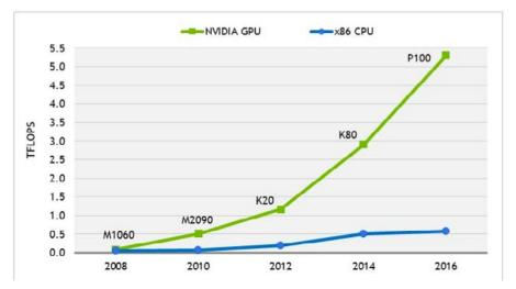
The latest generation of GPUs from NVIDIA contain upwards of 5,000 cores and deliver double-precision processing performance of 5 TeraFLOPS. Note also the relatively minor performance improvement over time for multi-core x86 CPUs, and how it is now flattening. (Source: NVIDIA)
